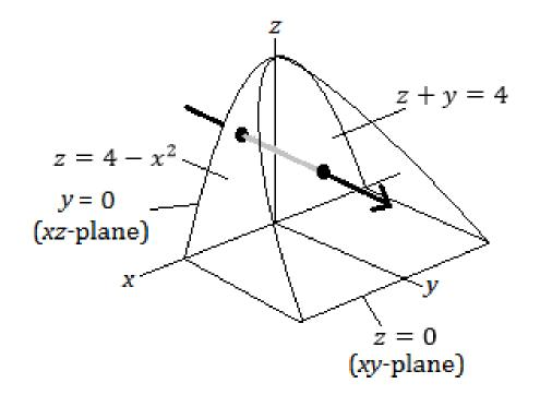
This arrow enters the solid at the *xz*-plane  $(y_1 = 0)$ , passes through the interior (gray), and exits out the plane z + y = 4, or  $y_2 = 4 - z$ . These are the bounds for y.
